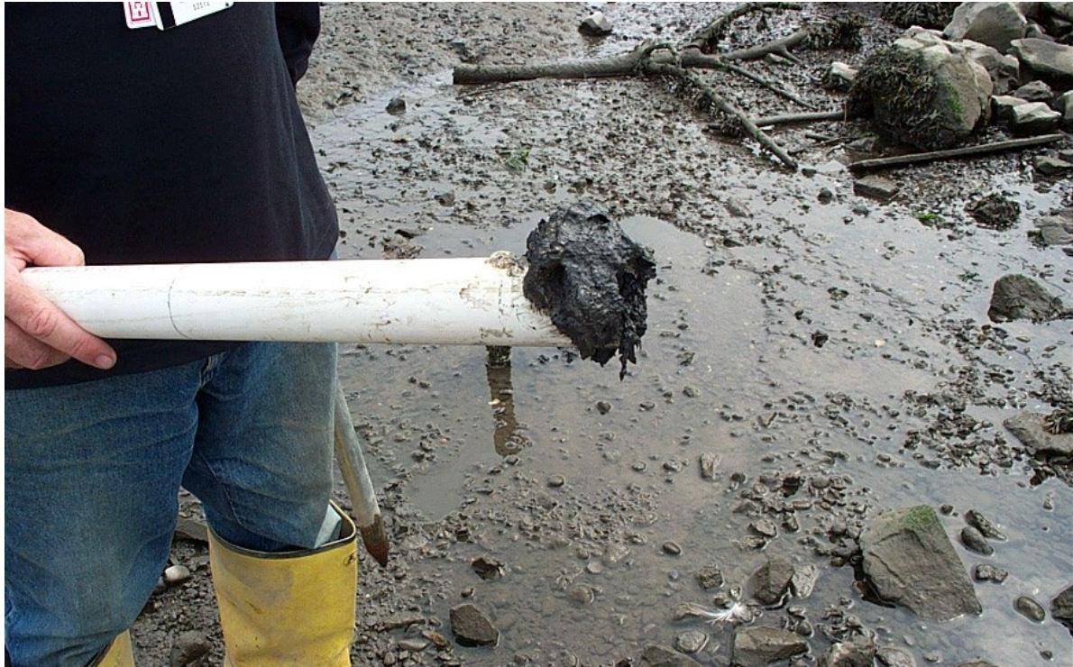
Figure 3.2. Black mud from beneath the tidal flat surface, consistent with the strongly reducing conditions indicated by low Eh and dissolved oxygen observations. (Durgin, 9/24/01).
