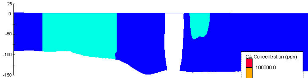
Figure 2.63. Initial CA profile along section B-B' (Fig. 2.29); with TCA DNAPL source within hot spot #3.
