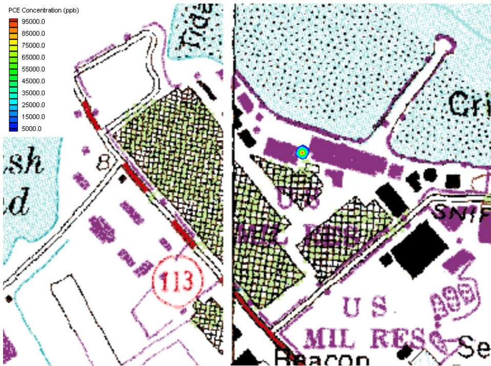
Figure 2.20. Predicted PCE distribution after 20 years; DNAPL source imposed in hot spot #2, within reworked glacial sediments (grid layer 3).
