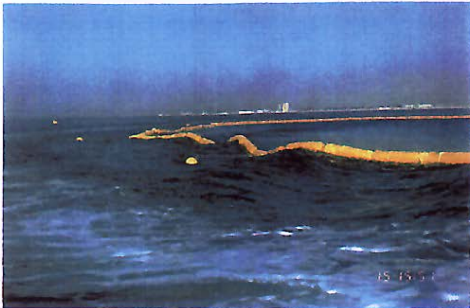
Photo 11: SeaCurtain Boom heave and roll response demonstration
