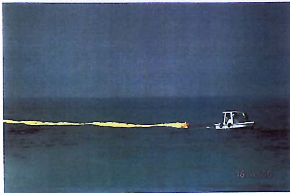
Photo 15: Towing SeaCurtain Boom towards shore for recovery
