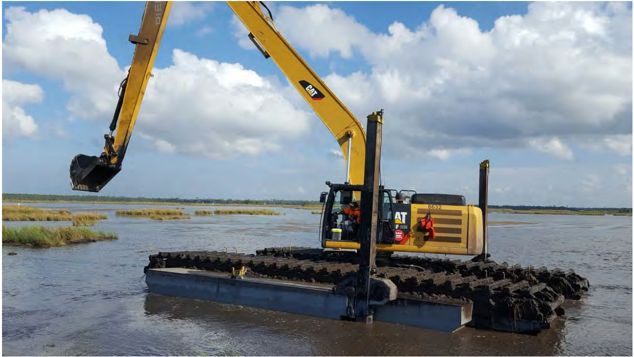
Figure 7. Alternative 4 – Amphibious Dredge - Mechanical. Source: BIG Dredging
