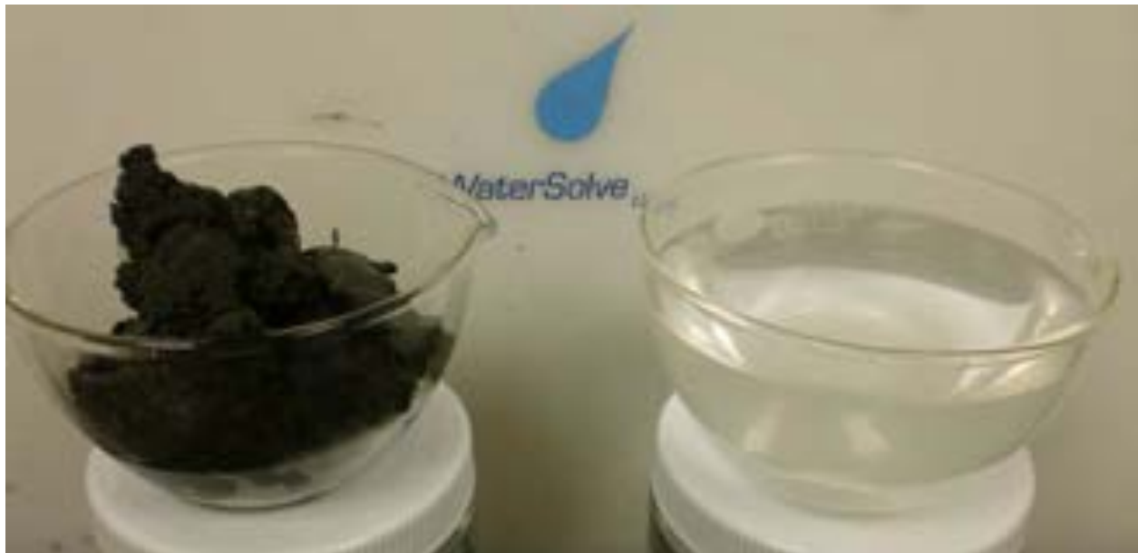
A one thousand milliliter sample conditioned with Solve 137 was poured through the GT500D Geotube® fabric. The captured cake (Left) and filtrate (Right) are shown above.
