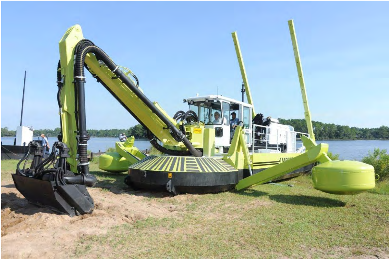
Figure 8. Alternative 4 – Amphibious Dredge - Mechanical. Source: Amphibex
