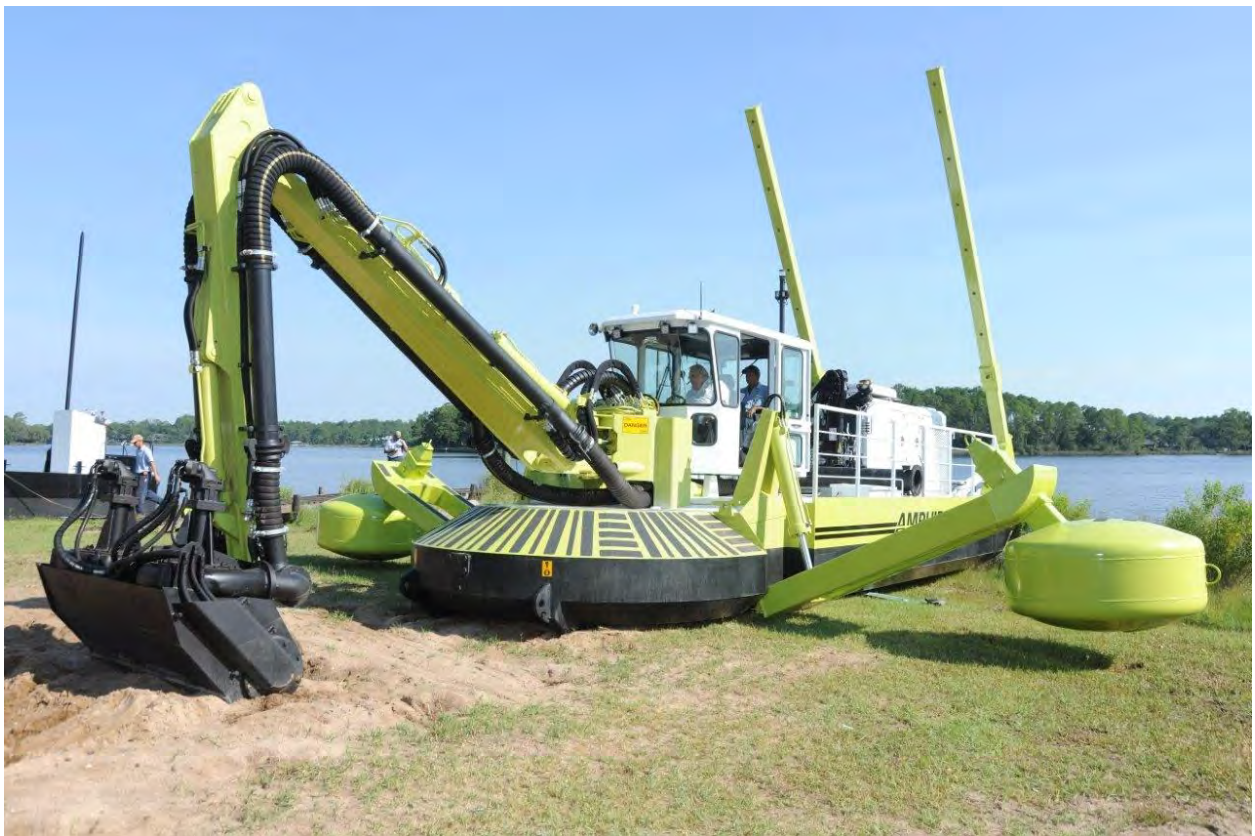
Figure 8. Alternative 4 – Amphibious Dredge - Mechanical. Source: Amphibex
